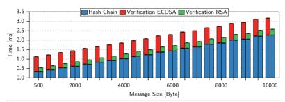
**Figure 5.15** The mean processing time required for verifying a control message with a verification interval of 20 and a group size of 1 scales roughly linearly with the payload size. This is mainly due to the effort required for verifying the correctness of the hash chain.
