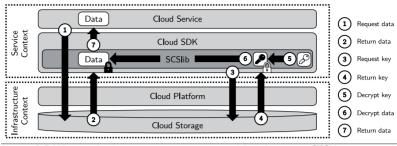
**Figure 5.5** When a cloud service requests a protected IoT data item, SCSlib transparently handles all necessary security operations, i.e., requesting necessary data protection keys from the cloud, verifying the digital signature, and decrypting individual data fields.
