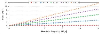
Figure 6.9 The network overhead generated by one user's ControlCenter scales linearly in the number of ControlCenters in the user's PriverCloud instance and the heartbeat frequency.
