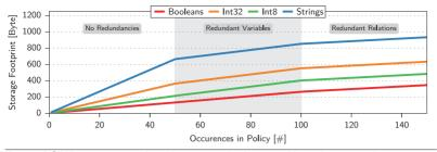
Figure 4.6 When increasing the policy size, redundant variables, relations, and integer optimization improve compression and hence reduce storage footprint.
