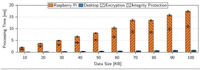
Figure 6.4 The overhead of PriverCloud's secure storage results from encryption as well as integrity protection and scales roughly linearly with increasing data size.
