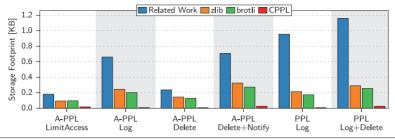
Figure 4.12 When considering real-world privacy policies, CPPL considerably reduces storage footprint compared to related work and generic compression methods.
