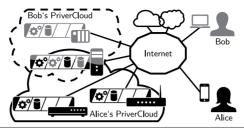
**Figure 6.1** In our envisioned scenario, each user builds her individual PriverCloud instance over trusted devices contributed by friends and family. A user can use processing ( $\Phi^{o}$ ) and storage (**1**) resources on these devices to realize Internet-accessible privacy-sensitive cloud services.
