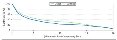
**Figure 3.25** The size of the anonymity set k directly influences the amount of contributions that can be utilized for comparison-based privacy. Buffering contributions for a day slightly increases the fraction of contributions that can be utilized.
