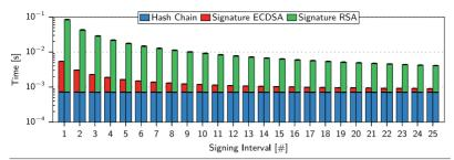
**Figure 5.12** The mean processing time for appending a message of length 2500 byte to the message log depends on the signing interval. Increasing the signing interval reduces the average time spend in the predominant signing operation.
