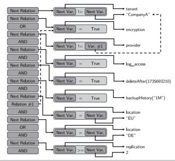
**Figure A.1** Decompression of a policy during evaluation at a cloud node. First, the algorithm iterates over the formula stack to find the beginning of the relations, thereby pushing elements of the formula stack onto an interpretation stack (left) which yields the policy in reverse polish notation. In a second step, the algorithm evaluates the policy based on the reverse polish notation, i.e., it resolves and evaluates relations and applies the boolean operations to the corresponding results.
