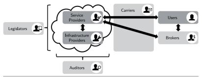
Figure 2.3 The cloud computing landscape consists of different actors and their relationships and interplay. We mark the three actors that are most important for privacy (from a technical perspective) and are hence in the focus of this dissertation in dark gray.
