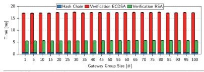
**Figure 5.16** The number of gateways that append control messages to the message log has a negligible impact on the mean processing time required for verifying one message of length 2500 byte in the message log with a verification interval of 20.
