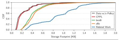
Figure 4.14 CPPL considerably reduces the storage footprint of real IoT data in the cloud compared to privacy policies from related work.
