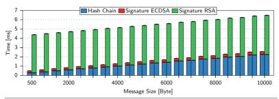
Figure 5.13 The mean processing time for appending a message of varying payload size to the message log with a signing interval of 20 and a group size of 1 increases roughly linearly with the payload size.
