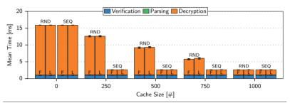
Figure 5.8 SCSlib's caching approach considerably reduces the overhead for processing protected IoT data in the cloud, both for random (RND) and especially sequential (SEQ) access to IoT data when using FIFO (F) and LRU (L) as cache management scheme.
