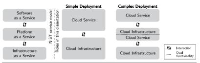
**Figure 2.2** Deviating from the NIST service model with IaaS, PaaS, and SaaS, in this dissertation, we differentiate cloud offers by their role into cloud infrastructure and cloud service. In a complex deployment, one cloud offer can act as both, cloud service and cloud infrastructure.
