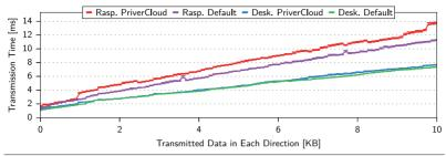
Figure 6.6 Using PriverCloud sockets adds a modest overhead for the transmission time required for communicating with a cloud service.
