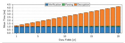
Figure 5.7 The mean time for processing one IoT data item for a key change interval of 10 and an unlimited cache size linearly increases with the number of data fields.
