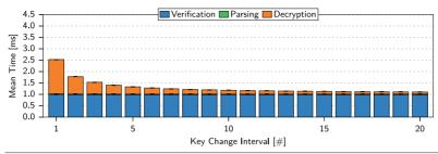
Figure 5.6 The mean time for processing one IoT data item with one data field for an unlimited cache size decreases with increasing key change intervals.
