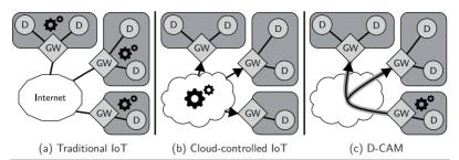
Figure 5.9 Different current IoT deployment models realize configuration, authorization, and management (a) within isolated IoT networks or (b) centrally in the cloud. In contrast, D-CAM (c) enables *distributed* control *across* network borders without having to trust the cloud.
