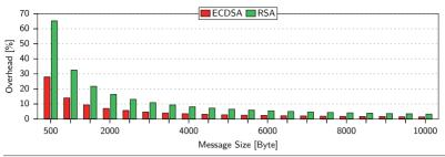
Figure 5.17 The relative per-message storage and communication overhead of D-CAM reduces with increasing message size.
