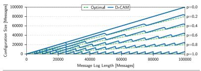
**Figure 5.18** The influence of trimming the message log depends on the probability of messages being obsoleted (p = 0, 0.2, ..., 1). D-CAM at most incurs a fixed overhead, whose precise value is a configurable parameter of D-CAM (here: trimming after 5000 obsolete messages).
