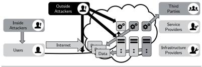
**Figure 2.6** Attacks that threaten privacy in cloud computing originate from a variety of internal (dark gray) as well as external (black) entities.
