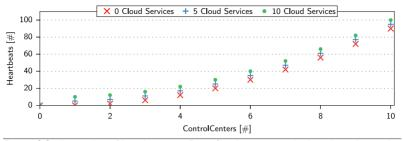
Figure 6.8 The number of heartbeats in a PriverCloud instance scales linearly in the number of deployed cloud services and exponentially in the number of backup ControlCenters.
