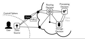
Figure 4.3 When data leaves the control sphere of the user, per-data item policies empower her to still influence routing, processing, and storage decisions.
