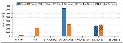
**Figure 6.7** The time required for deploying a cloud service in a PriverCloud instance amounts to about 1s and predominantly results from remote attestation and starting the cloud service within a secure execution environment.
