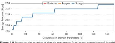
Figure 4.9 Increasing the number of domain parameters (and hence expressiveness) logarithmically increases the storage footprint.
