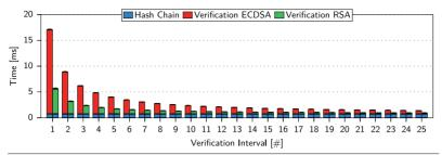
**Figure 5.14** The mean processing time for verifying one control message of size 2500 byte in the message log depends on the verification interval. By increasing this interval, the average time spent for the predominant operation for verifying the digital signature is reduced.
